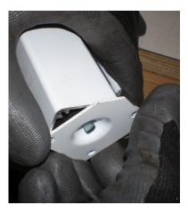
Insert square pin into mounting hole of housing end cap, rotate cap clockwise wind up spring. Add 15—18 turns. KEEP a good gripe so spring won't release. *Gloves are recommended*.
